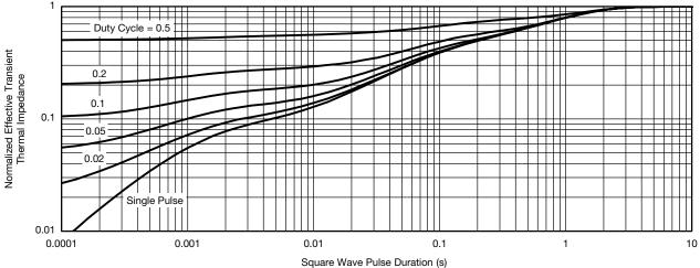
Normalized Thermal Transient Impedance, Junction-to-Foot
