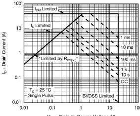
$V_{DS} \text{ - Drain-to-Source Voltage (V)} \\ ^*V_{GS} \text{ > minimum } V_{GS} \text{ at which } R_{DS(on)} \text{ is specified}$
