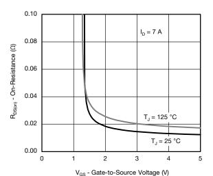
On-Resistance vs. Gate-to-Source Voltage
