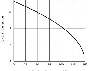
T<sub>C</sub> - Case Temperature (°C) **Current Derating\***
