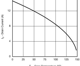
T<sub>C</sub> - Case Temperature (°C) **Current Derating\***
