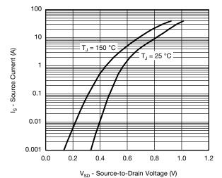
Source-Drain Diode Forward Voltage
