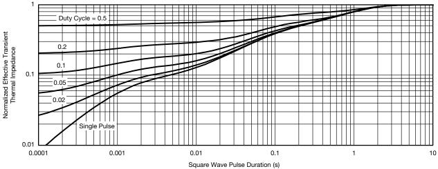
Normalized Thermal Transient Impedance, Junction-to-Foot
