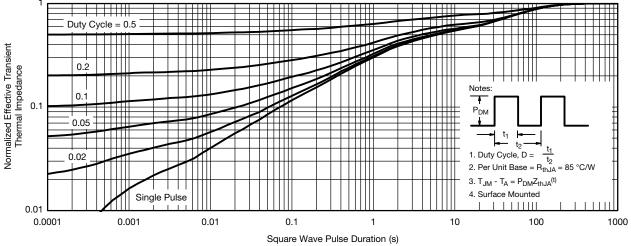
Normalized Thermal Transient Impedance, Junction-to-Ambient
