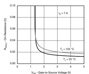
On-Resistance vs. Gate-to-Source Voltage
