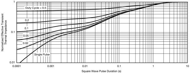
Normalized Thermal Transient Impedance, Junction-to-Foot
