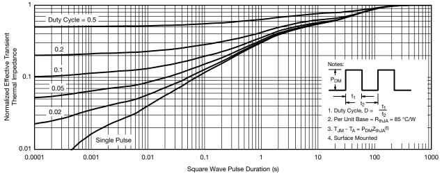
Normalized Thermal Transient Impedance, Junction-to-Ambient
