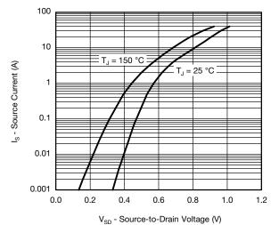
Source-Drain Diode Forward Voltage
