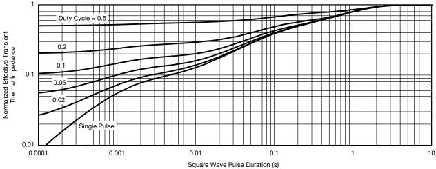
Normalized Thermal Transient Impedance, Junction-to-Foot
