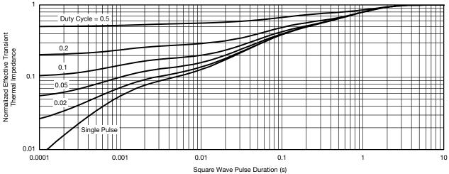
Normalized Thermal Transient Impedance, Junction-to-Foot
