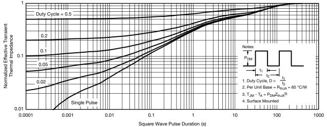
Normalized Thermal Transient Impedance, Junction-to-Ambient
