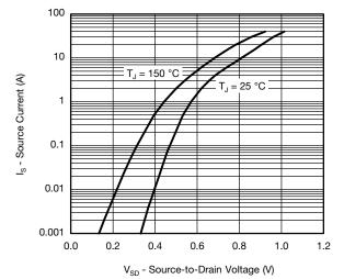
Source-Drain Diode Forward Voltage
