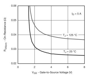
On-Resistance vs. Gate-to-Source Voltage
