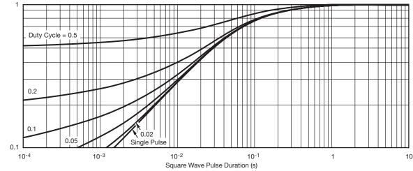
Normalized Thermal Transient Impedance, Junction-to-Foot
