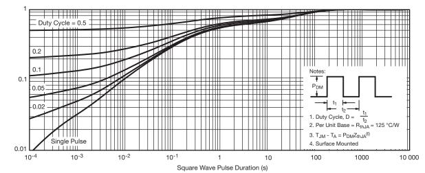
Normalized Thermal Transient Impedance, Junction-to-Ambient
