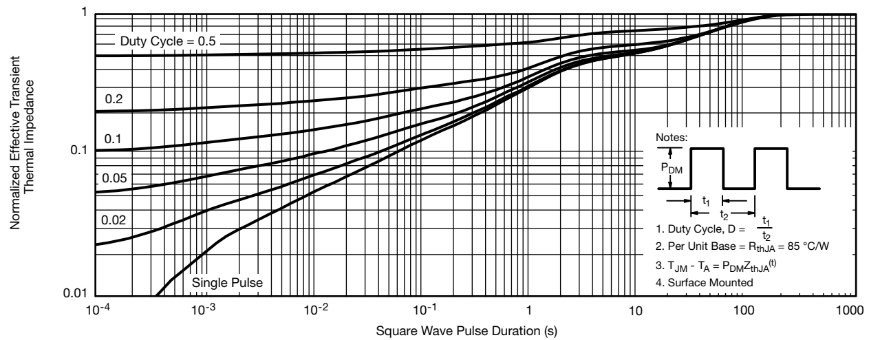
Normalized Thermal Transient Impedance, Junction-to-Ambient
