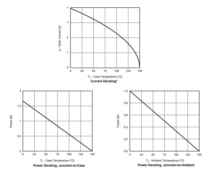
\* The power dissipation  $P_D$  is based on  $T_{J(max)}$  = 150 °C, using junction-to-case thermal resistance, and is more useful in settling the upper dissipation limit for cases where additional heatsinking is used. It is used to determine the current rating, when this rating falls below the package limit.
